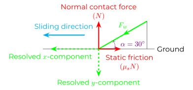
As shown in the diagrams above, decreasing the angle of the skate to the ground ( $\alpha$ ) decreases the normal contact force (N) and increases the horizontal component (x-component) of the force of the wheels on the ground ( $F_w$ ).
