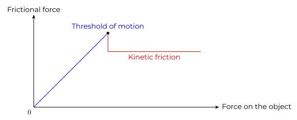
Remember static friction increasing as the force on the object increases from section 2.5? (The graph is also shown above for easy reference.) That is exactly why the force of the wheels on the ground should be minimised. This minimising of force on the wheels on the ground is usually only applicable to the preparation phase of a slide, which is when you would bend or sit lower to enter the slide.
