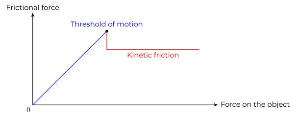
As you can see from the graph above, static friction increases as the force on the object increases until the threshold of motion, then it decreases and remains constant as kinetic friction. Keep this graph in mind, as it will be important later.
