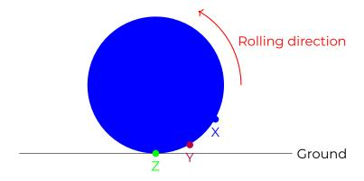
From the series of images above, you can tell that point X is never in motion, and it doesn't move. Instead, as the wheel rolls, point X rolls away and is no longer in contact with the ground. Every second, a new point comes into contact with the ground, which is point Y at t=2 and point Z at t=3. Hence, since the points are not moving when they are in contact with the ground, the friction we should consider is static friction. Thus, we consider the static friction in the case of rolling.
